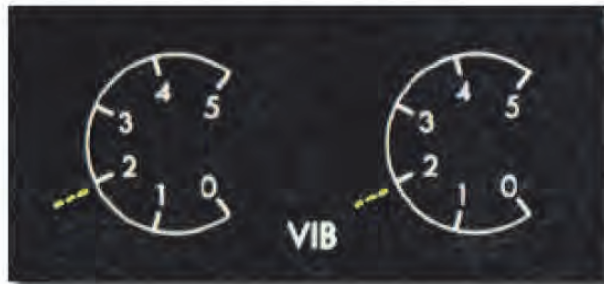
Figure 2-69: Vibration indicator dials of later version of Boeing 737. Source: UK Air Accidents Investigation Branch.
