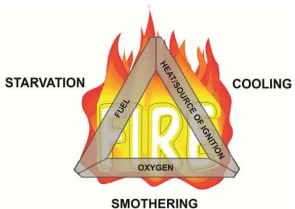
Figure C2-8: The fire triangle. Source: CorelDraw! 5.0 clipart.
